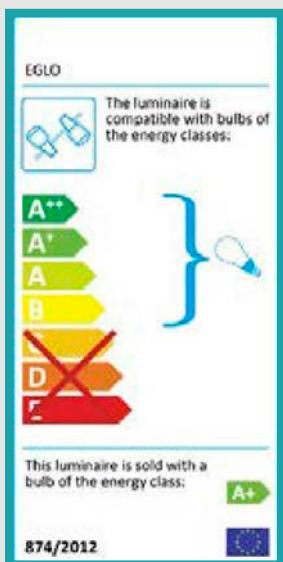
The information in brackets at the centre of the label indicates which bulbs may be used for the luminaire. In this case, the product is only compatible with bulbs with an energy efficiency rating of better than C.
