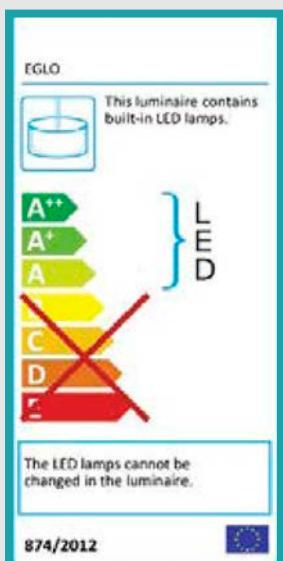
This label indicates that the luminaire is sold with built-in LED lamps that cannot be replaced by the consumer himself.
